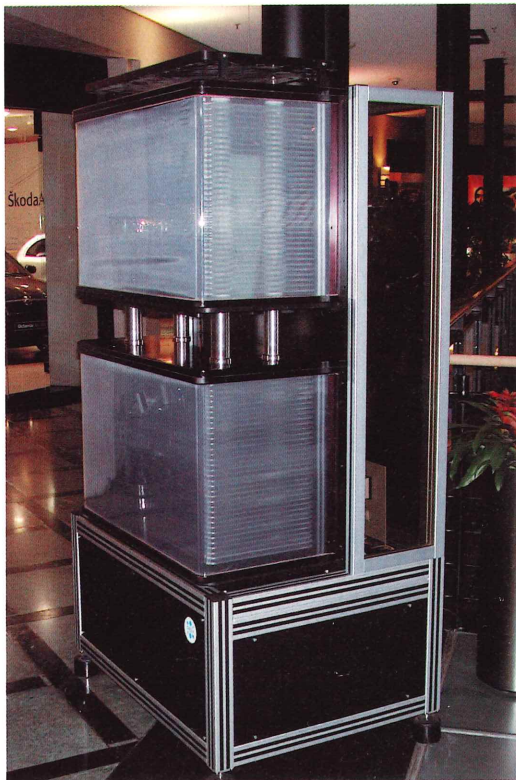
Spark Chamber / built in 1999 / metal, Plexiglas electronic / 79 x 43.3 x 31.4" / weight 700 kg / Zeuthen, DESY Instrument to produce proof of cosmic radiation
